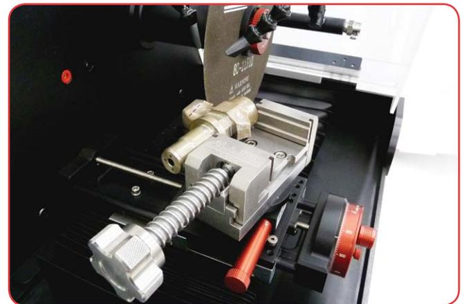
The fixture rotation stage (shown with #5-5525 vise) allows angle cutting in 2° increments. A variety of fixtures can be mounted to provide rotational adjustment of the sample relative to the blade. It mounts directly to the indexing tables or Z-axis stage.
