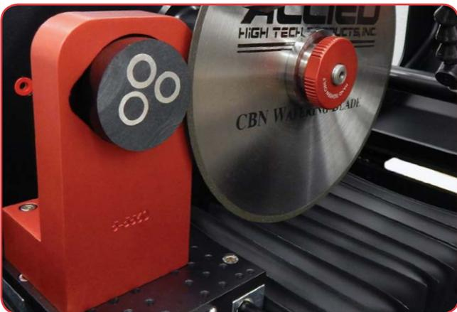
The teardrop holder secures various sized mounts from 25 mm to 2" diameter. It is mounted to the indexing tables for precise location sectioning, and positions the mount at the center of the blade.
