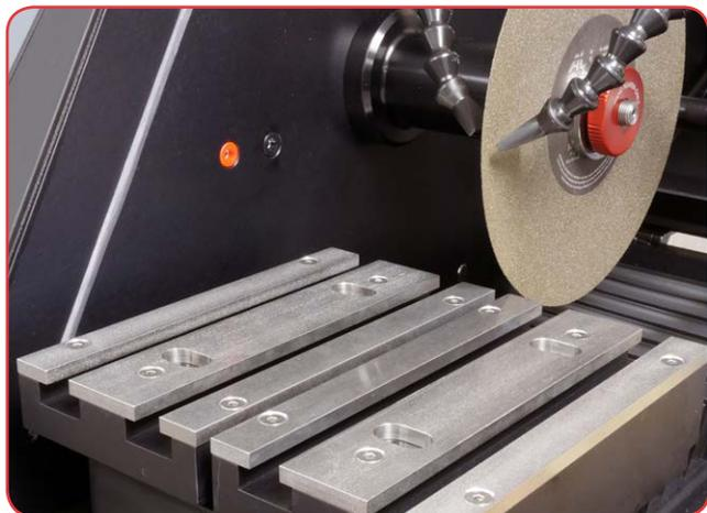
The T-slot table allows a wide range of clamping and fixturing options available to accommodate a variety of sample shapes and sizes.
