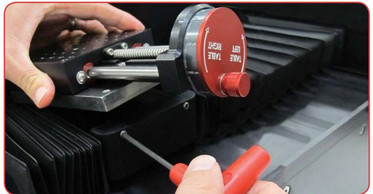
The TechCut 5's unique design allows the use of either a T-slot table or X-axis indexing table, which are easily and quickly changed to support a wide range of fixture configurations.
