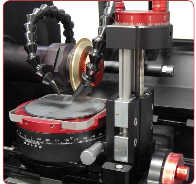
The dicing rotation stage (shown mounted on #5-5730 Z-axis stage and #5-5325 fine indexing table) allows 360° rotational positioning of flat substrates. Samples are mounted to the borosilicate glass insert using wax, which is secured with set-screws for quick attachment and removal. It can be mounted directly to the indexing tables, or to the Z-stage to control cutting depth.
