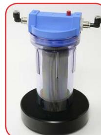
With a reusable/cleanable 75 µm stainless steel filter, this filtration system is designed for applications where excessive debris is generated during sectioning operations (plastics, resins, composites, ferrous metals).
