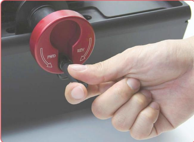
Manual Y-axis sample advancement using the hand wheel provides additional flexibility in positioning and feeding. The wheel is utilized to slowly feed delicate samples into the blade for minimal damage, allowing the user to "feel" the sectioning operation or to quickly position the sample prior to sectioning. It is also convenient for blade dressing.
